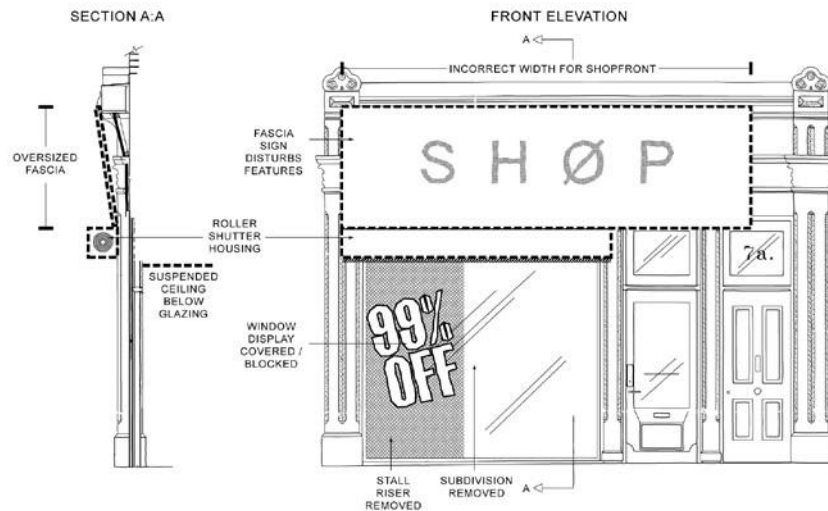
Figure 10. Inappropriate shopfront section and elevation
