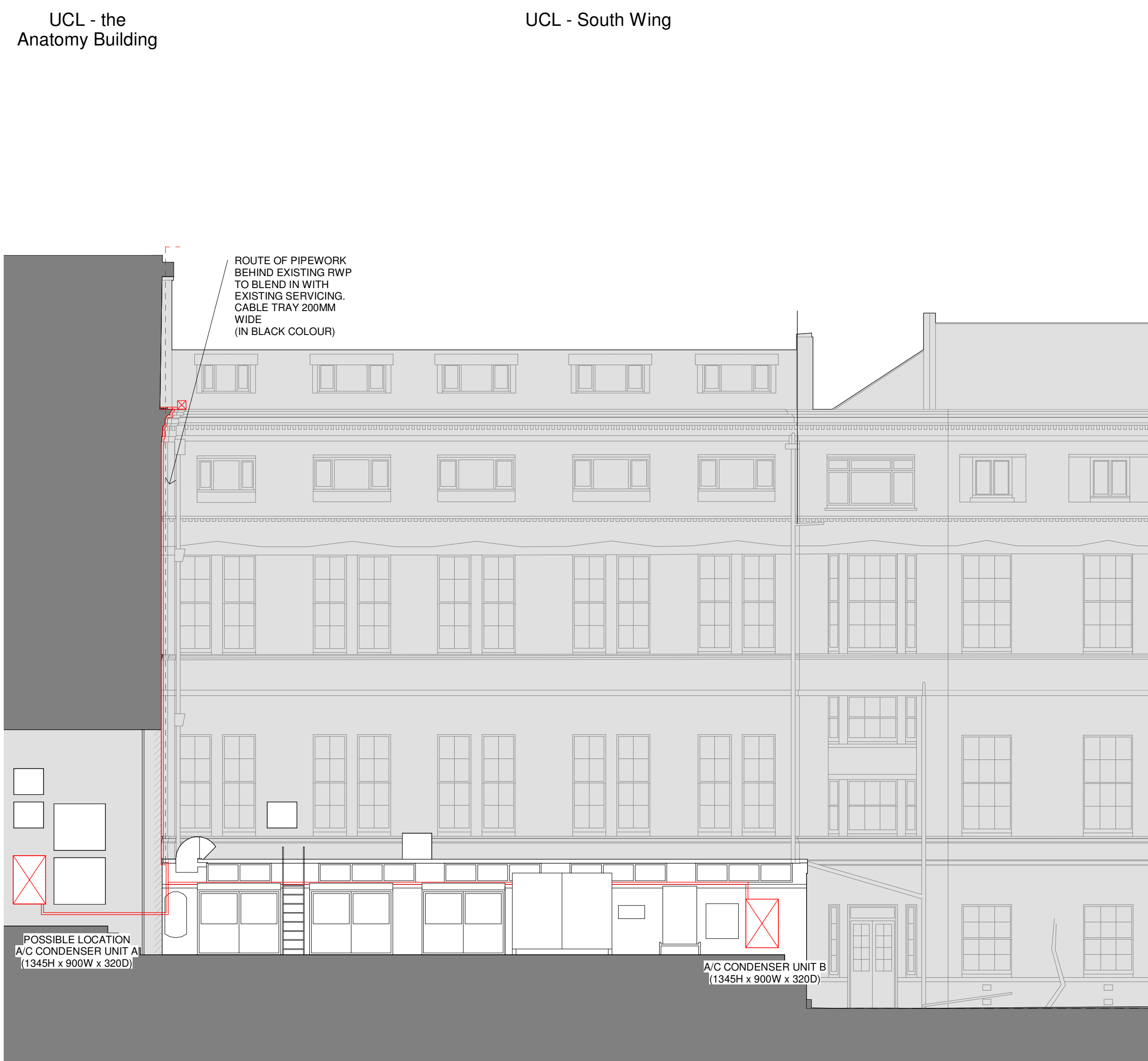
Proposed Section AA' - New External A/C Plant 1 : 100
