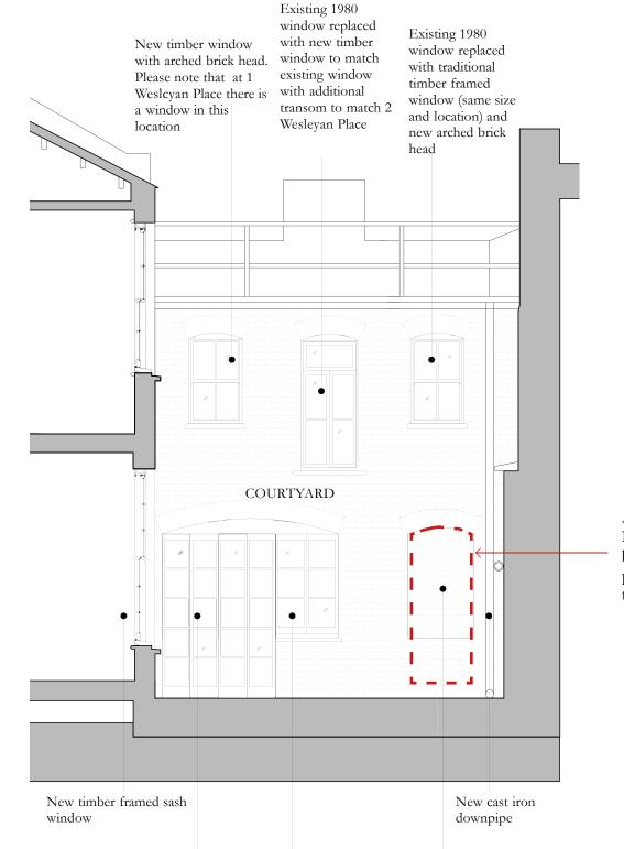
Area in dotted line is the only new brickwork. New brickwork to toothed into adjacent brickwork, in the same bond as existing and painted white to match surrounding elevation.
