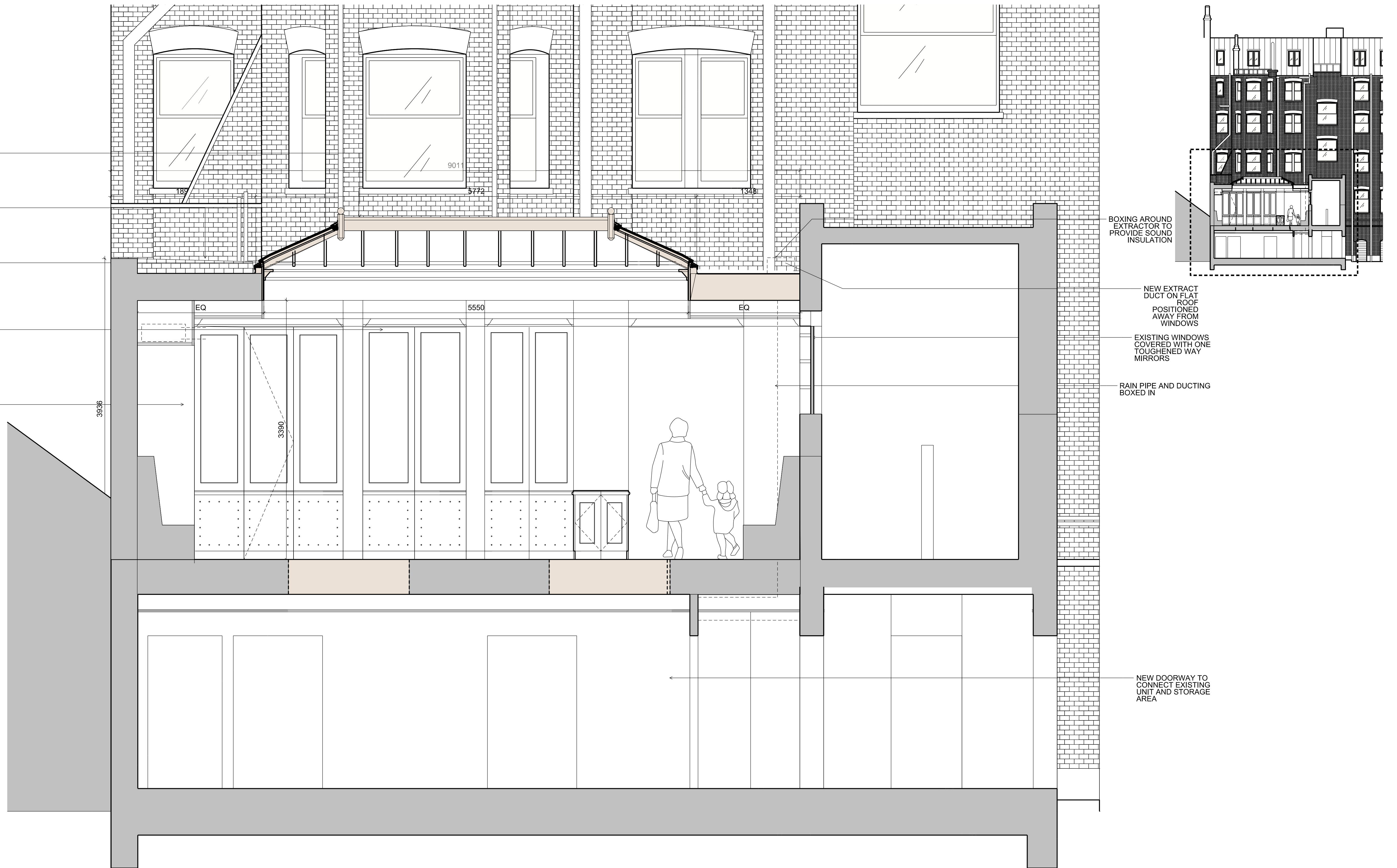
01 PROPOSED SECTION AA DETAIL 1:50
