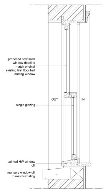
Proposed second floor half landing new sash window - Section
