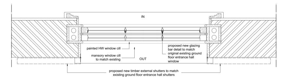
Proposed ground floor drawing room new sash window -Plan
