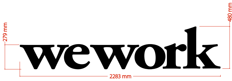
Sign 3 - 1 Set of Built up non-illuminated aluminium letters fixed above windows (2 Sets Black)
