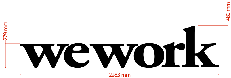
Sign 1 - 1 Set of Black built up non-illuminated aluminium letters fixed above windows
