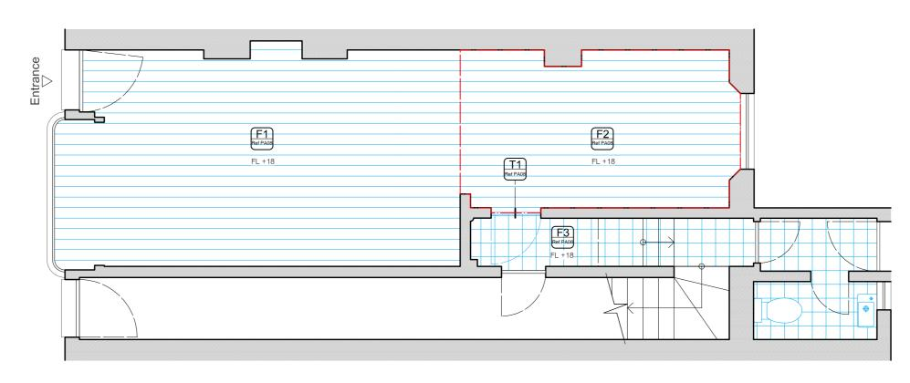
Antique Engineered Oak Size: 190x1900x15 Finish: Oiled and distressed with black dye Supplier: Flooring365 Tel: 03330020175 Note: to be install on ten of the existing floor tiles with underlay (floating floor) See detail: F1, PA08
