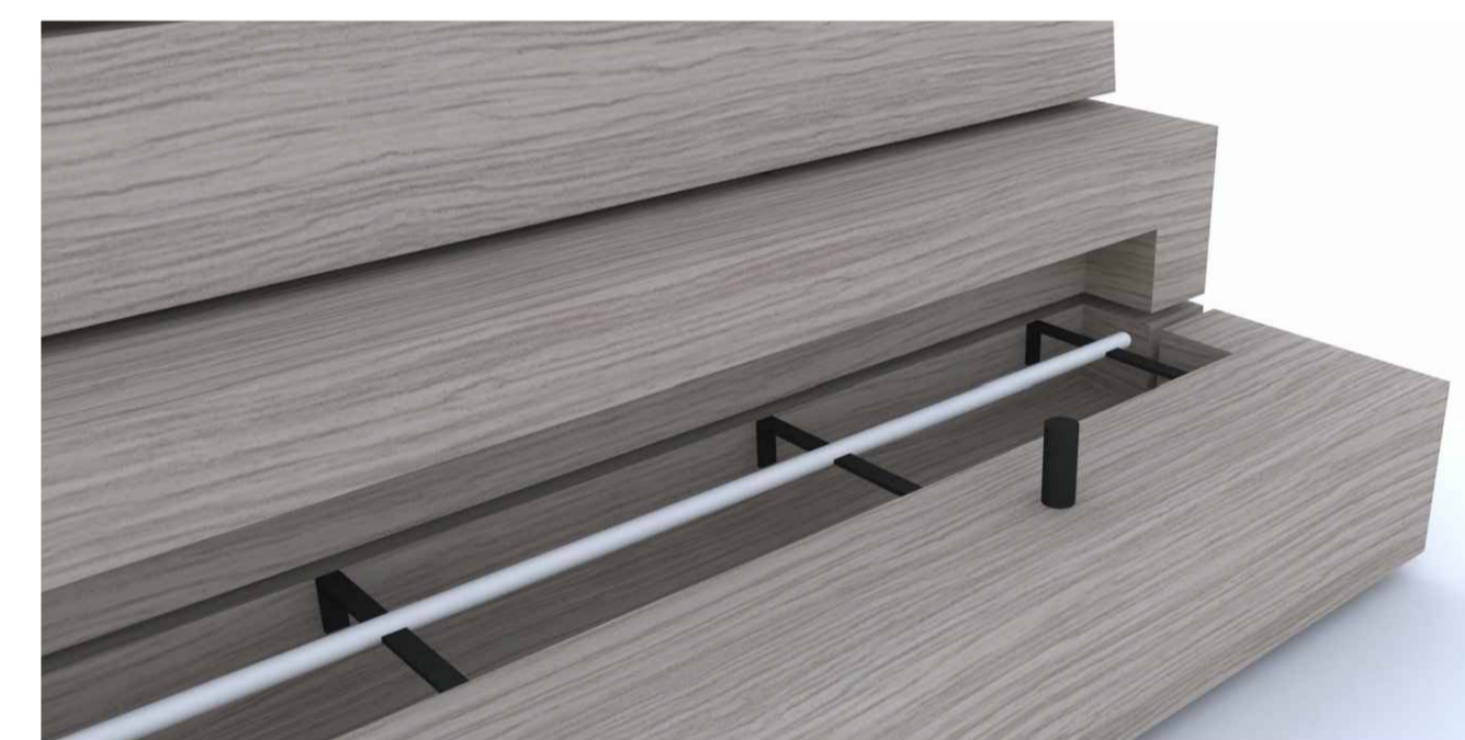
ILLUSTRATIVE VIEW OF BESPOKE ILLUMINATED TIMBER BENCH WITH BACK INTERNAL LED STRIP LIGHT
