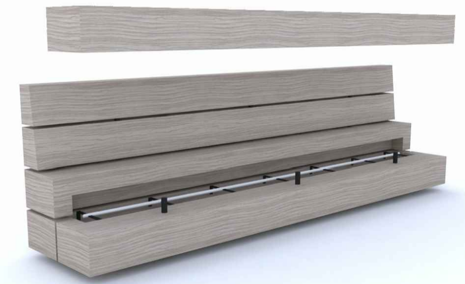
ILLUSTRATIVE VIEW OF BESPOKE ILLUMINATED TIMBER BENCH WITH BACK REMOVABLE TOP TIMBER MEMBER
