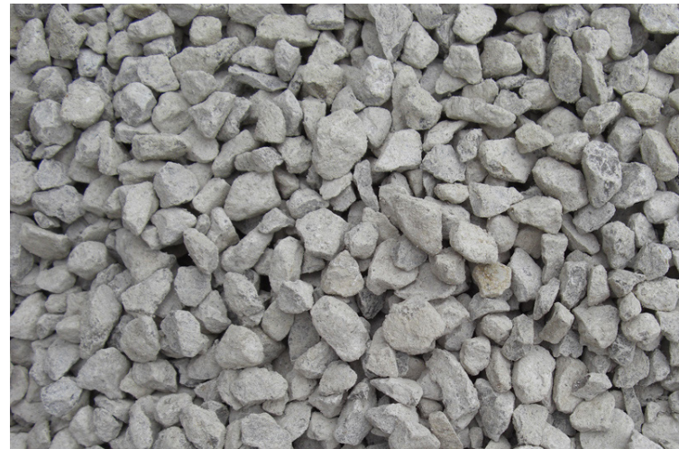
02 | Cell reinforced stone chippings
