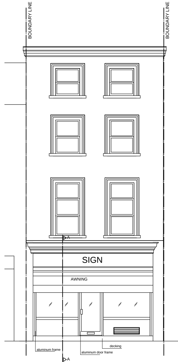
EXISTING FRONT ELEVATION WITH AWNING SCALE: 1/100 @ A3
