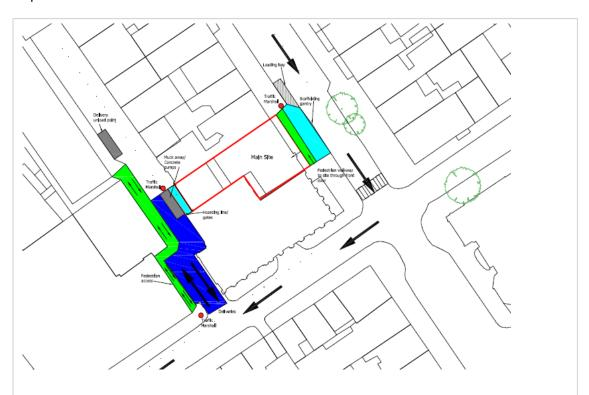
To minimise disruption with McGees down Tottenham Mews who have the road closed we will be converting the car park bays to a loading bay. Traffic marshals will control the pubic during large deliveries, these will be lifted onto the gantry scaffold and brought onto site. Smaller deliveries can be walked through the front entrance on the ground floor.
