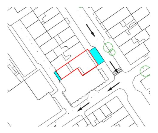
The shaded area illustrates the extent of the scaffolding, the scaffolding will bridge over the existing cycle rack that are on the path.
