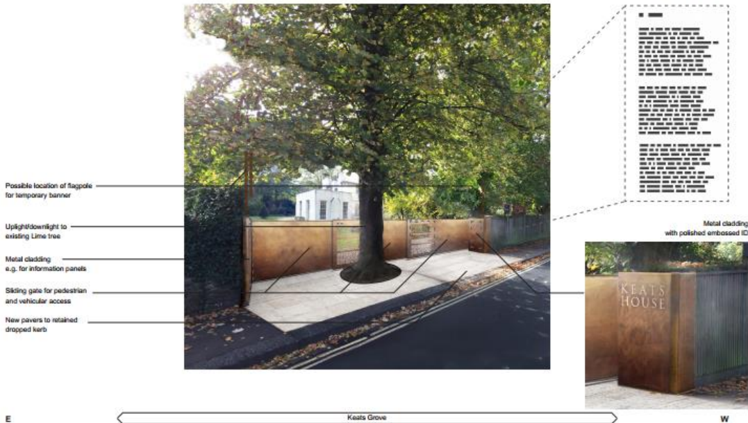
Fig. 6) Proposed entrance from Keats Grove. Proposed entrance steps back, improving the setting at the existing line tree. Signage is minimal. Enclosure (e.g. for security) is retained and some permeability to allow views and light through. The material proposed is a dark "autumnal" colour, referring to "To Autumn" poem by Keats, as well as being subtle and robust. The perforations are created from cutting out the words of the same poem 'to autumn' see top right of image figs 9-11.
