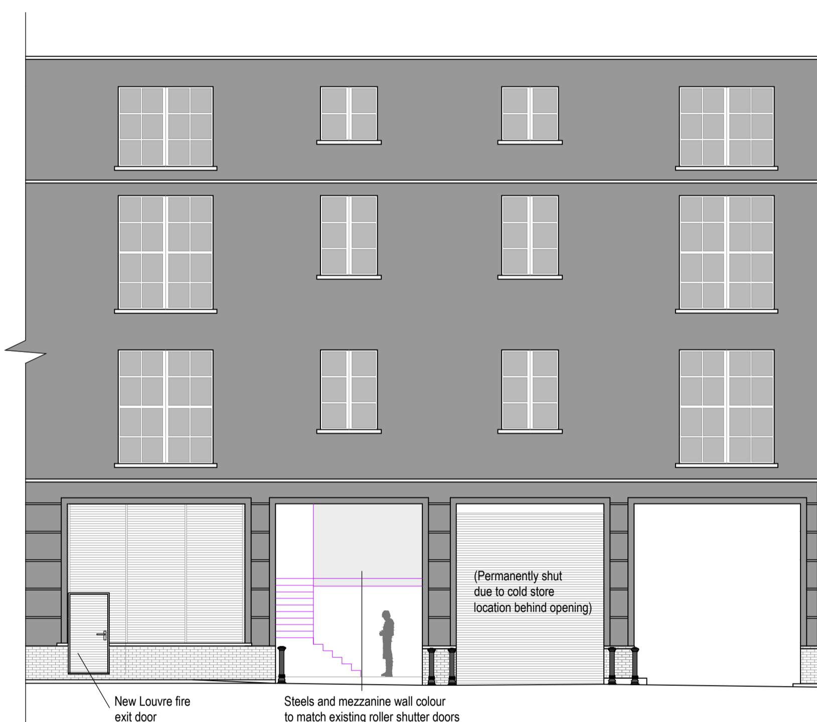
Proposed Rear Elevation (Showing Mezzanine Internally)
