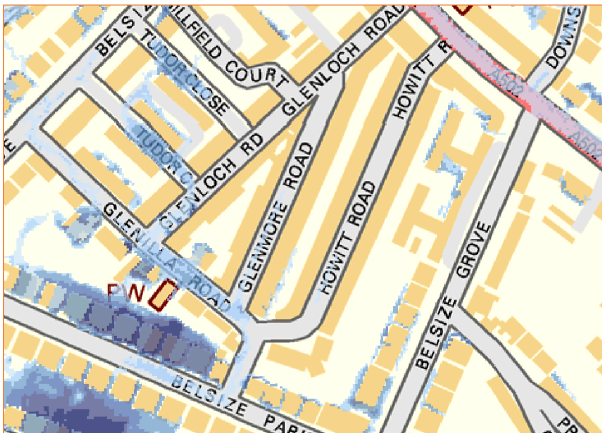
Figure 9: 1:1000 year pluvial flood depth mapping (Source: EA)
