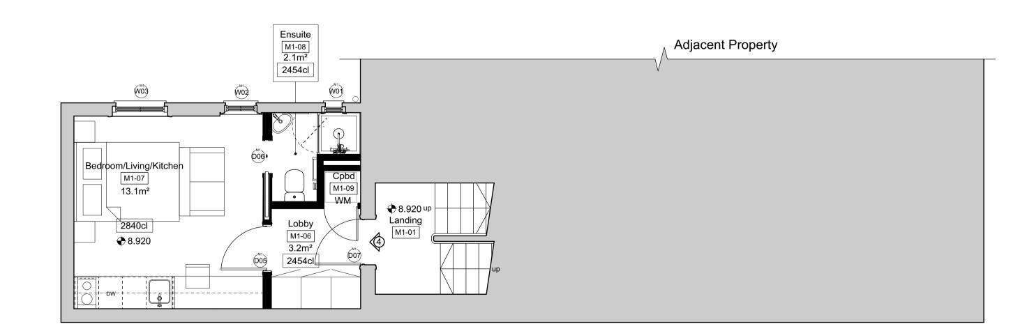
4 Proposed Mezzanine Floor Plan 1:100 @ A3 Unit 4: 20m2, Studio/2P DO NOT SCALE: Use figured dimensions only. All dimesnions are to be checked on site. Any queries or discrepancies must be reported immediately to the architect.
