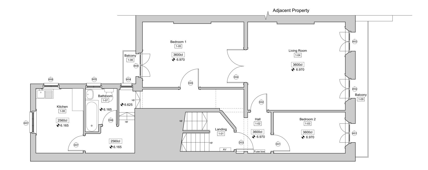
3 Existing First Floor Plan Scale: 1:50
