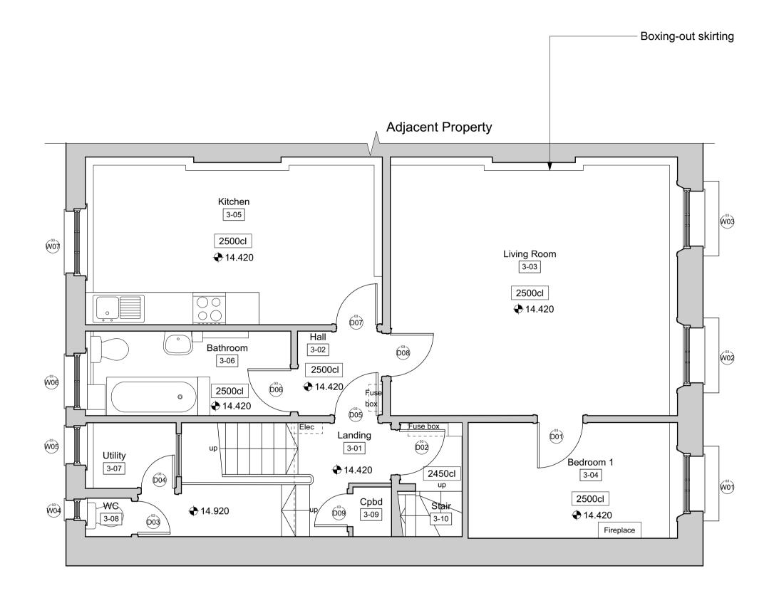
2 Existing Third Floor Plan Scale: 1:50 DO NOT SCALE: Use figured dimensions only. All dimesnions are to be checked on site. Any queries or discrepancies must be reported immediately to the architect.
