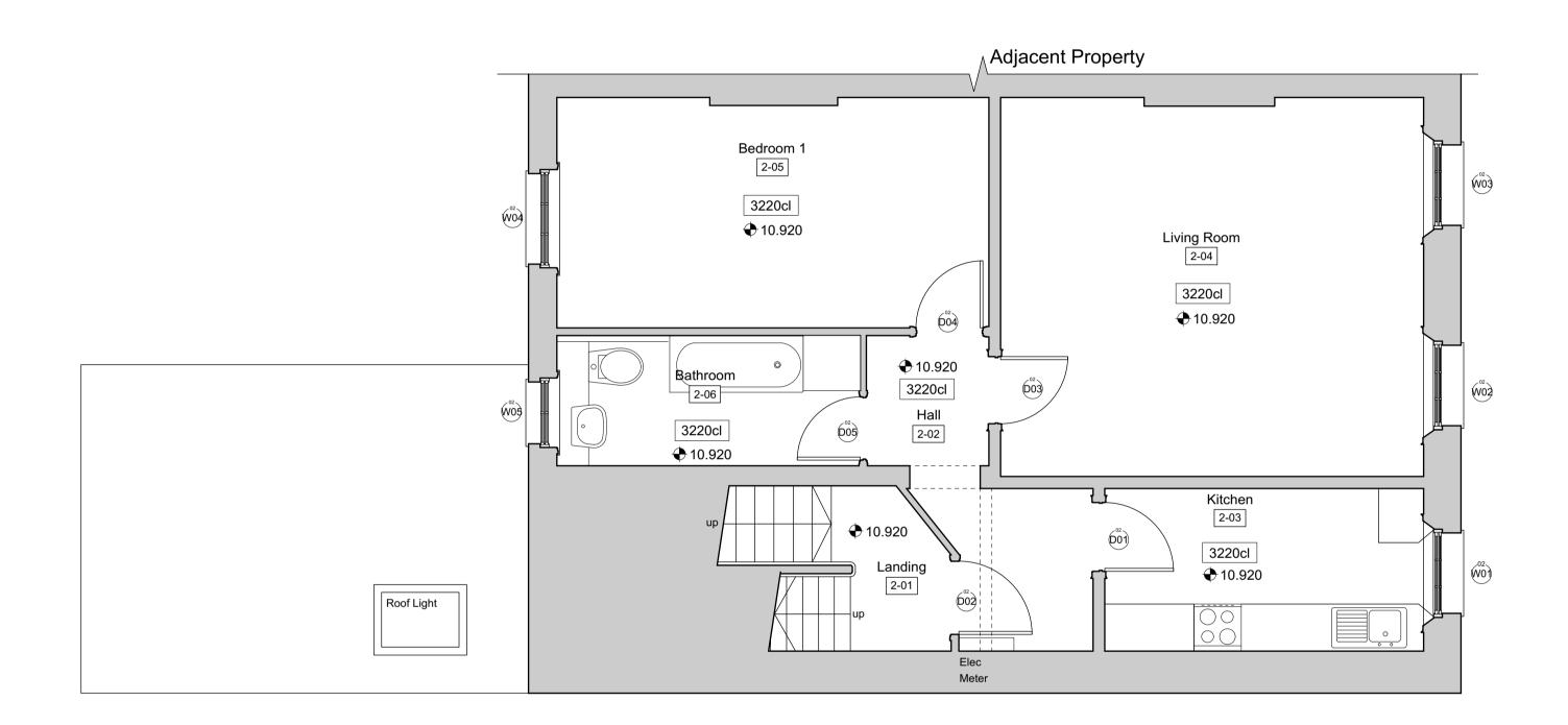
4 Existing Second Floor Plan Scale: 1:50
