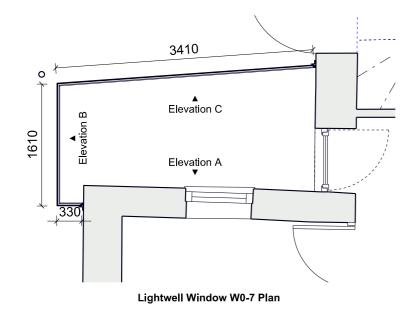
Structural Glazing: Structural Glazing shown indicatively. Structural glazing to achieve a minimum U Value of 0.16W/m2K in accordance with Part L1B of the Building Regulations. Glazing to be designed by Cantifix. Subdivisions and details to be checked and confirmed by architect prior to construction. Glass to be back painted at junction with ground floor to suit.
