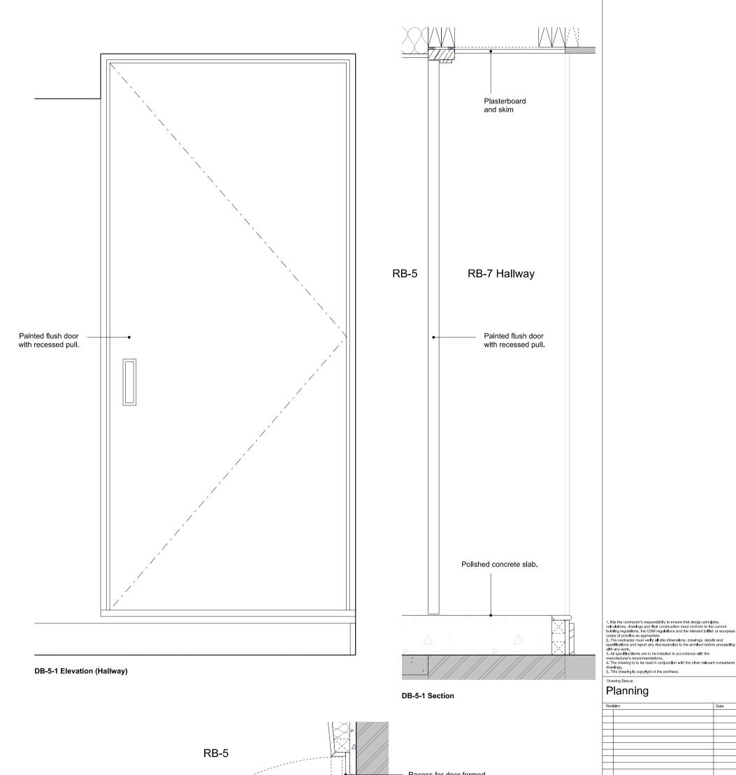
Recess for door formed with plasterboard and skim.
