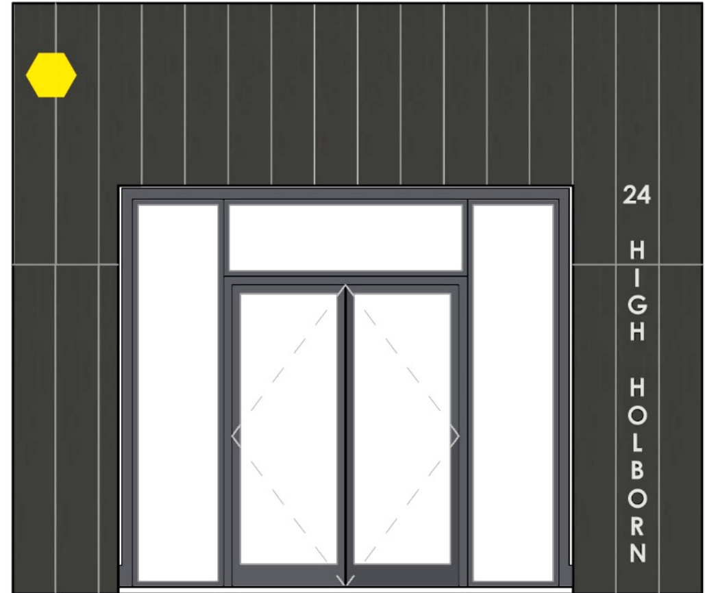
Visual reference showing proposed external fibre cement panel cladding, brushed stainless steel signage and fully glazed entrance doors with anthracite metal framing
