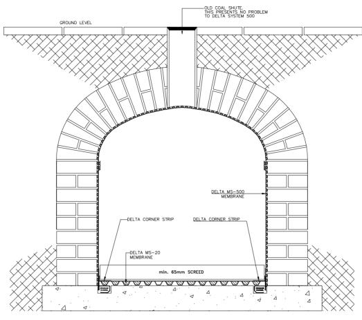
VAULTS CAN BE COMPLETELY SEALED AGAINST WATER INGRESS. EVEN RUNNING WATER PROBLEMS CAN BE CONTROLLED WITH MINOR MODIFICATIONS TO THE SPECIFICATION. THE SYSTEM CAN BE DRY LINED TO A DECORATIVE FINISH. THE FLOOR CAN BE SCREEDED OR FINISHED IN WOOD BASED SHEETS. WHERE A PLASTER FINISH IS REQUIRED, DELITA-PT CAN BE USED/SEEK ADVICE FROM OUR TECHNICAL DEPARTMENT.)
