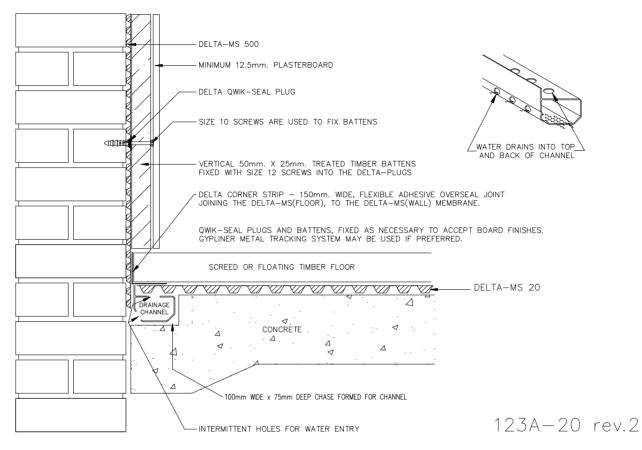
TYPE C, DRAINED PROTECTION, WALL AND FLOOR APPLICATION
