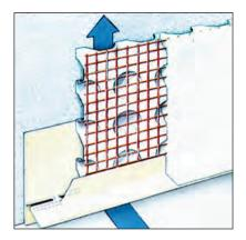
Ventilation gaps located at both top and bottom of the system allow circulation for this purpose.
