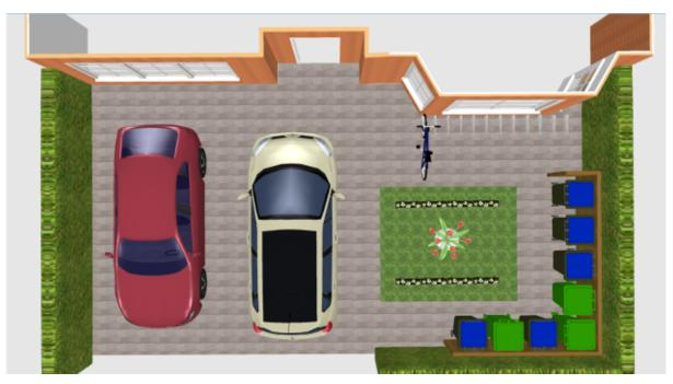
12. Waste storage will be as shown on the drawing as per item 11, which will be enclosed with timber.
