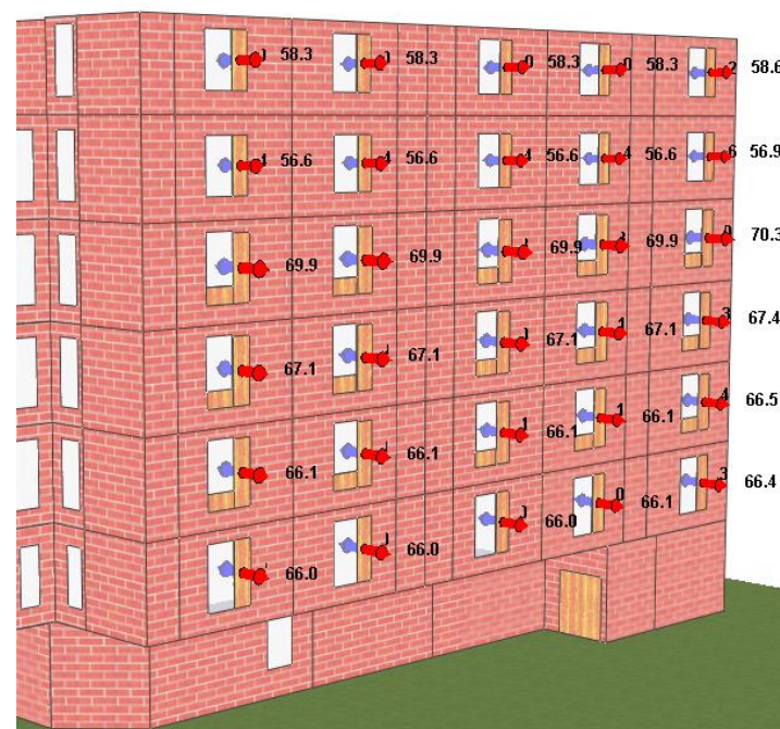
Figure 4.1 to show the air flow rates due to the natural ventilation of bedrooms
