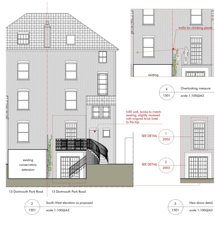
Revision Release date Drawn/Checked NOTES A 17/12/2018 CB First issue for planning PROJECT 15 Dartmout Simons-Dobson Avalon Construction & Design a: Black Mews, Richmond TW9 3GA e architecture@avalonbuild.co.uk ADDRES Comments from planning : infill brick wall insted of new window increase height of trellis from 1,20 m to 1,50 (as per neighbour comment); London - N B 26/02/2019 CB w avalonbuild.co.uk Test t:020 7348 9058 m:07891 174552 AVALON ACD 09181501
