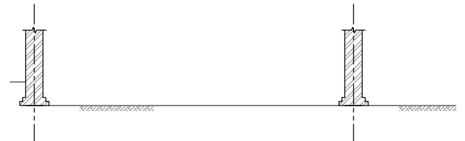
2. REMOVE EXTG FLOOR STRUCTURE & EXCAVATE TOPSOIL TO LVL OF EXTG FOOTINGS.
