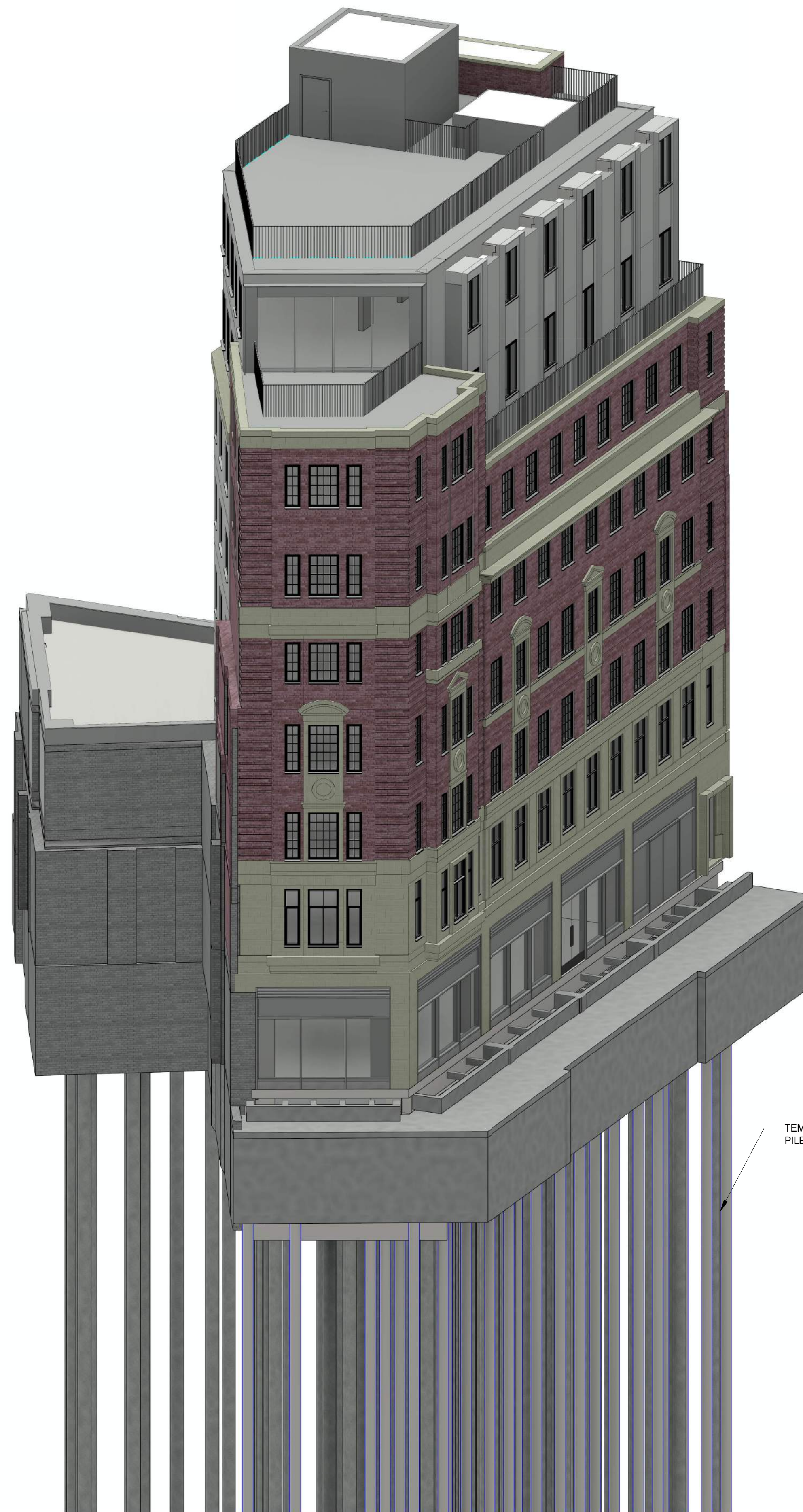
6 3D VIEW - TEMPORARY WORKS - SEQUENCE 6 TEMPORARY WORKS REMOVED.
