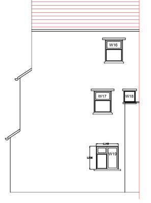
Existing windows are a mix of single glazed and double glazed timber and UPVC sash and casement windows to be replaced.
