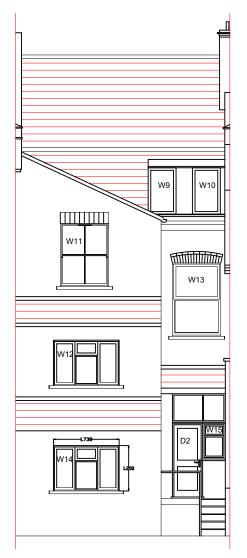
Existing windows are a mix of single glazed and double glazed timber and UPVC sash and casement windows to be replaced.
