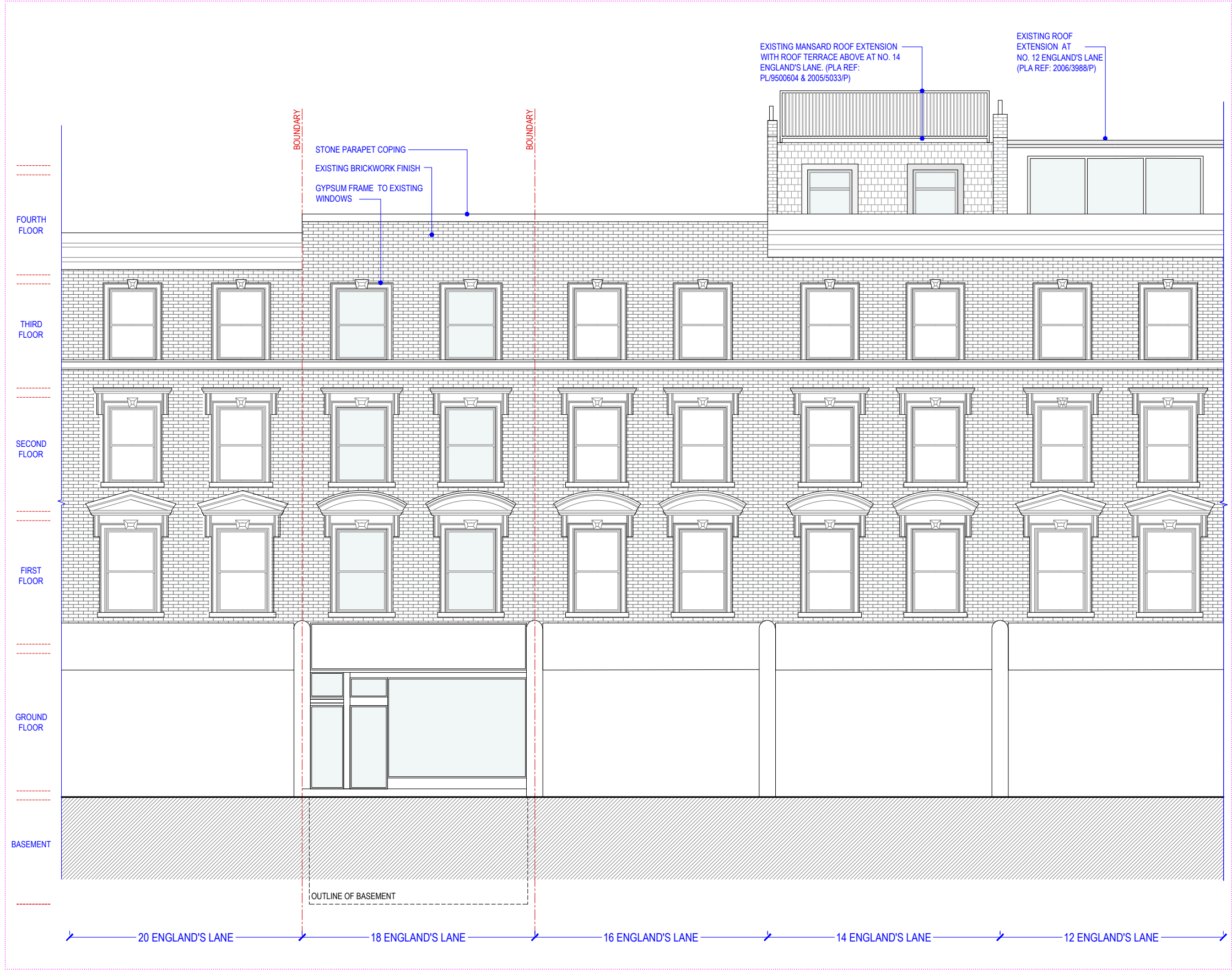
[01] EXISTING FRONT ELEVATION @1:100
