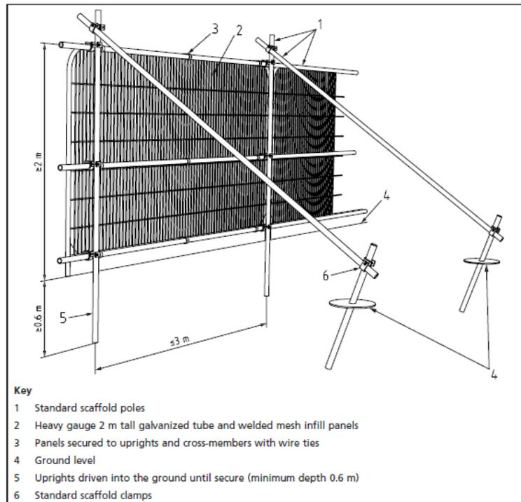
Fig. 1 Tree Protection Barrier Specification
