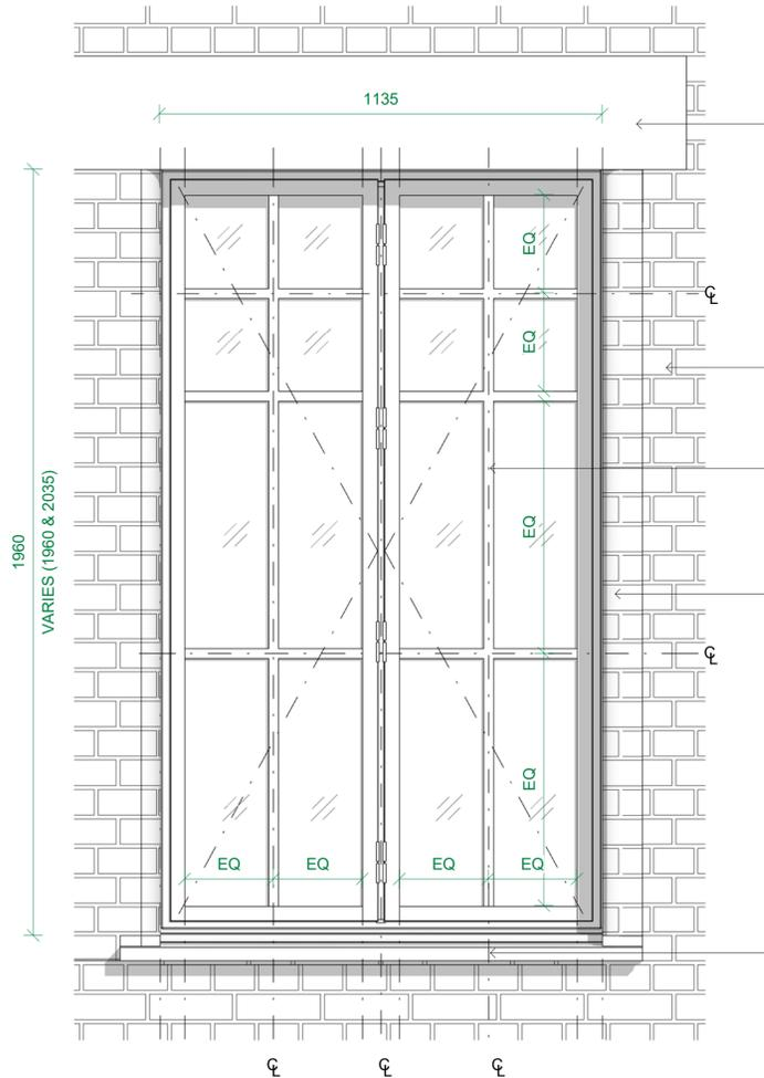
2 21 Denmark Place - Level 01-03 Typical AOV Elevation
