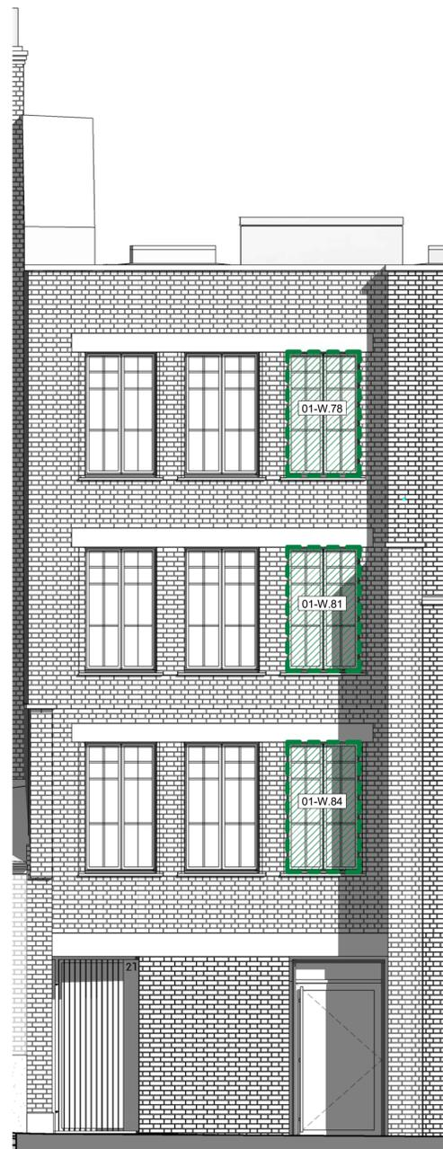
1 21 Denmark Place - Front Elevation - Level 01-03 AOVs
