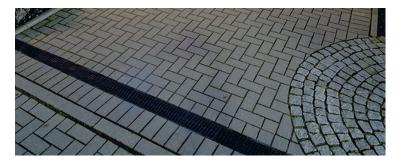
ACO HexDrain B 125 is suitable for vehicle traffic up to Load Class B 125, with soakaway crates below
