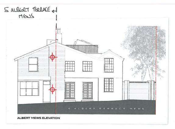
WE PROPOSE TO MONITOR THE FRONT& REAR ELEVATIONS AND THE PARTY WALLS FORTNIGHTLY DURING THE UNDERPINNING WORKS AND 6 WEEKS AFTER COMPLETION WE PROPOSE THE RED AND AMBER TRIGGER LEVELS TO BE:
