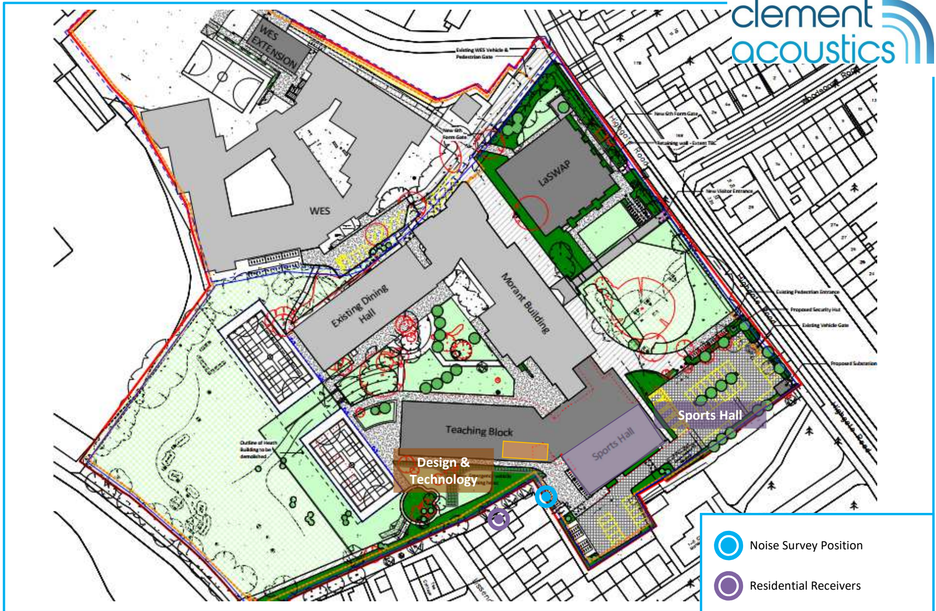
10883-SP1 Indicative site plan indicating noise monitoring position and nearest noise sensitive receivers
