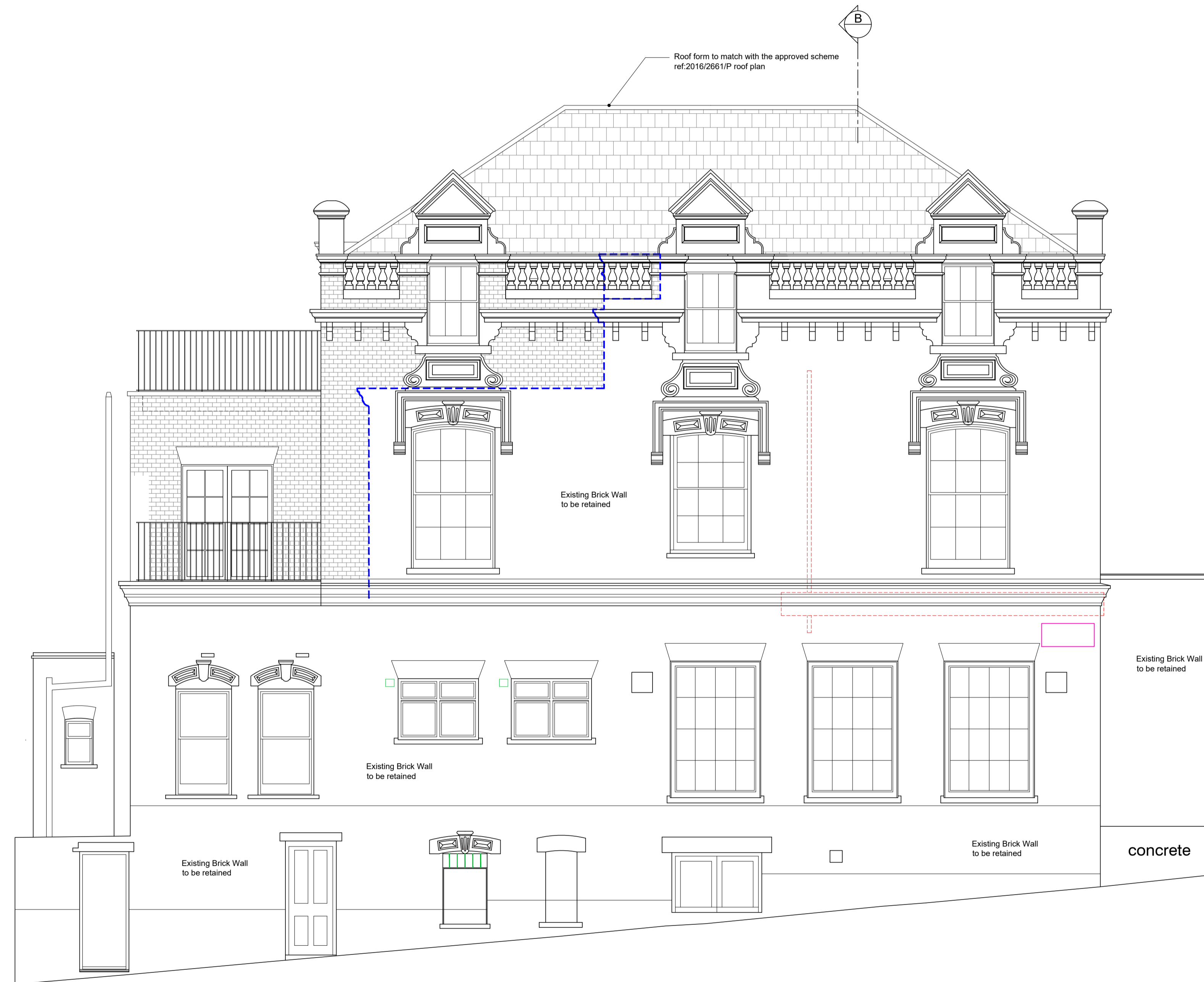
1 Existing Elevation 2 at Ravenshaw Street (Under Construction) as approved scheme ref:2016/2661/P
