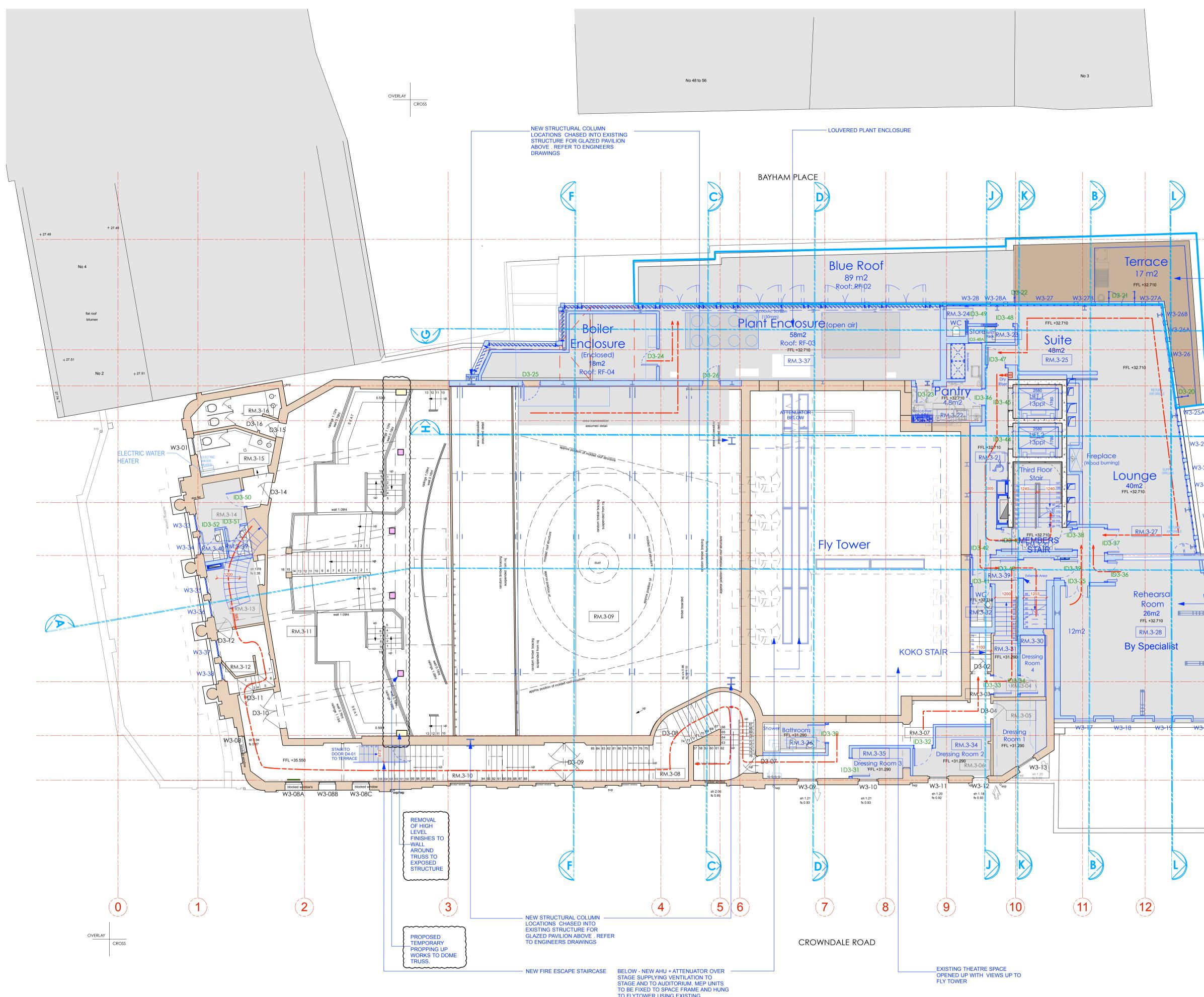
STAGE SUPPLYING VENTILATION TO STAGE AND TO AUDITORIUM. MEP UNITS TO BE FIXED TO SPACE FRAME AND HUNG TO FLYTOWER USING EXISTING RELOCATED SECONDARY STEEL BEAMS . REFER TO STRUCTURAL ENGINEER'S DETAILS, FLYTOWER TIMBER REPORT BY SPECIALIST AND DETAILS FROM EXTREME RIGGING.
