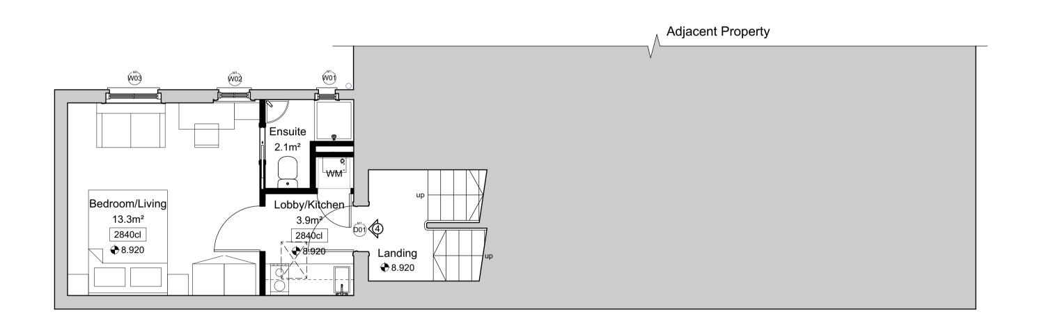
1 Proposed Mezzanine Floor Plan 1:100 @ A3 Unit 4: 20m2, Studio/2P DO NOT SCALE: Use figured dimensions only. All dimesnions are to be checked on site. Any queries or discrepancies must be reported immediately to the architect.
