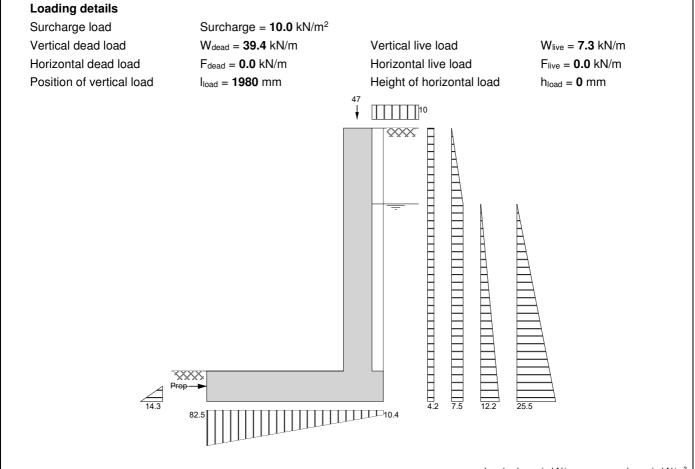
Loads shown in kN/m, pressures shown in kN/m<sup>2</sup>
