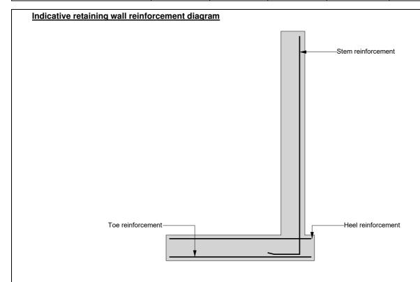
Toe bars - 16 mm dia.@ 125 mm centres - (1608  $\text{mm}^2/\text{m}$ )
