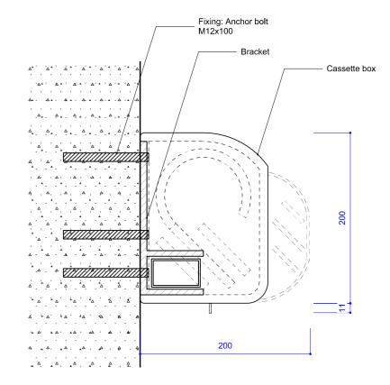
Fixing Point Elevation S=1/25 @ A3
