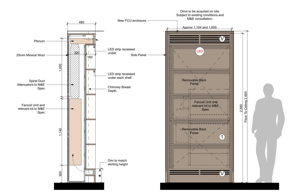
**S01** - Level LG Typical FCU Enclosure Section 1:20@A1
