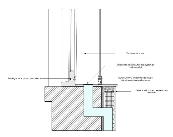
TYPICAL SECONDARY GLAZING DETAIL TO POOL AREA
