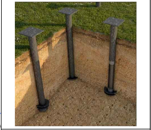
3D exposed cross sectional representation of screw pile foundations.
