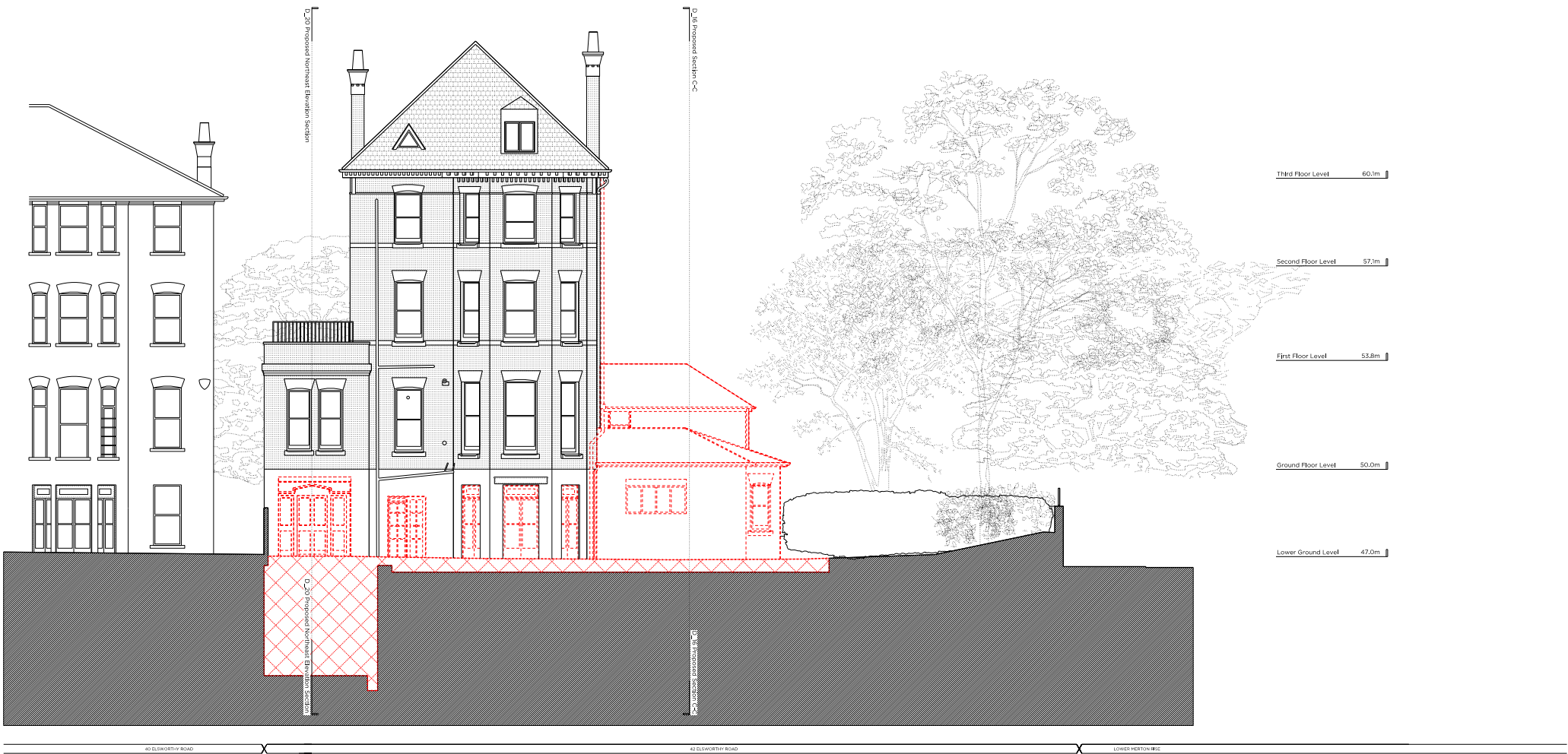
Demolition Northwest Elevation
