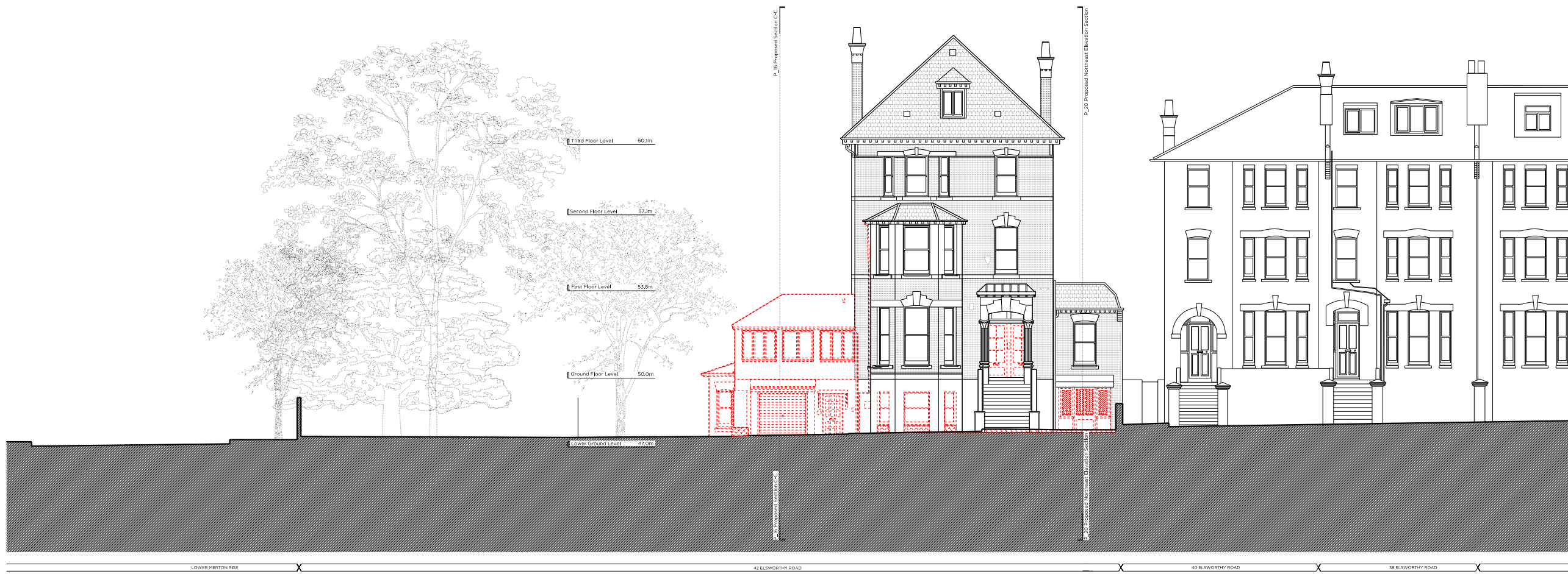
Demolition Southeast Elevation
