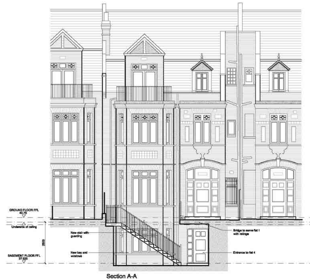
Proposed front elevation showing basement facade
