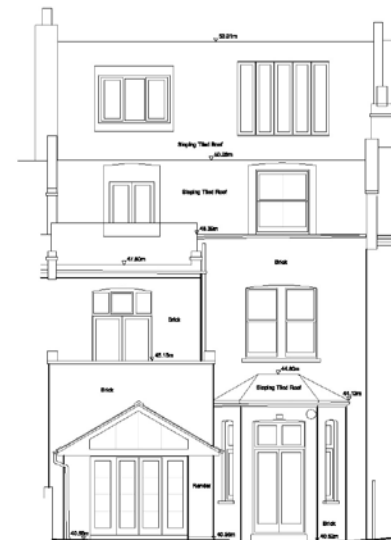
Rear facade survey
