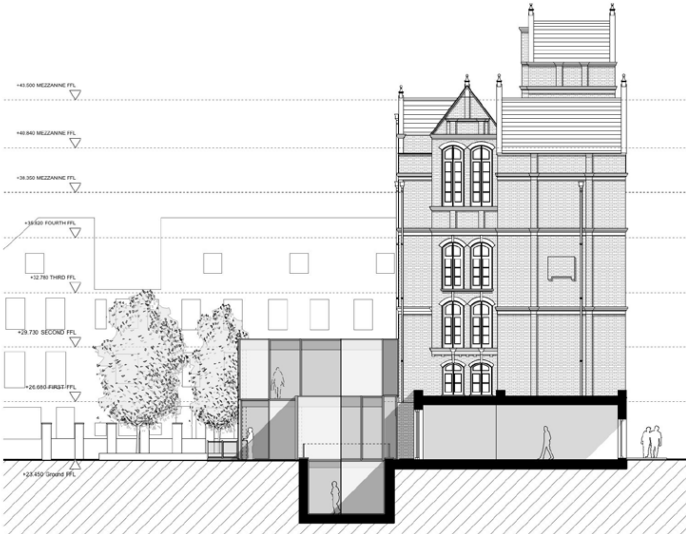
Drawing submitted as part of the 2014 application, showing proposed 2 storey rear extension and basement
