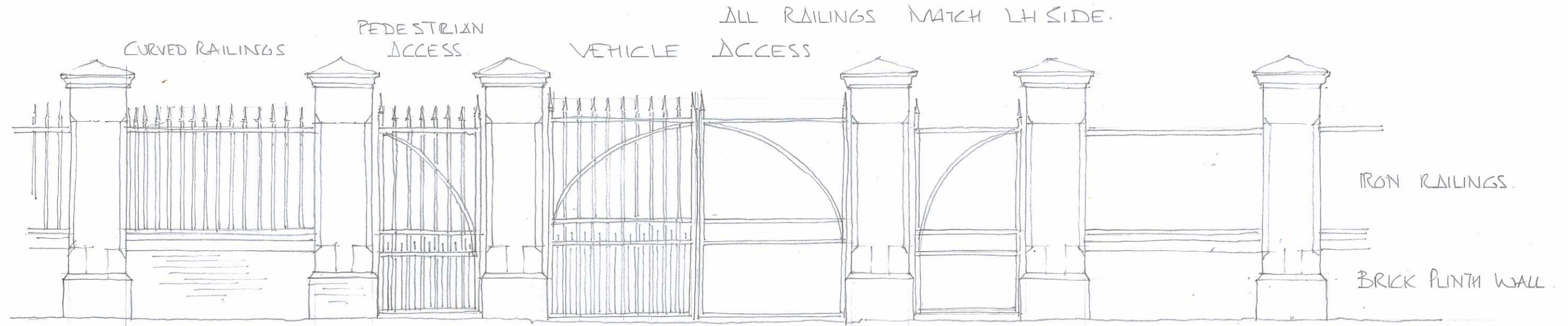
ELEVATION AS EXISTING
